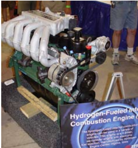
While this may look like a normal internal combustion engine, it is not. This engine was adapted for hydrogen fuel use by the Hydrogen Engine Center of Argonne, Iowa.
