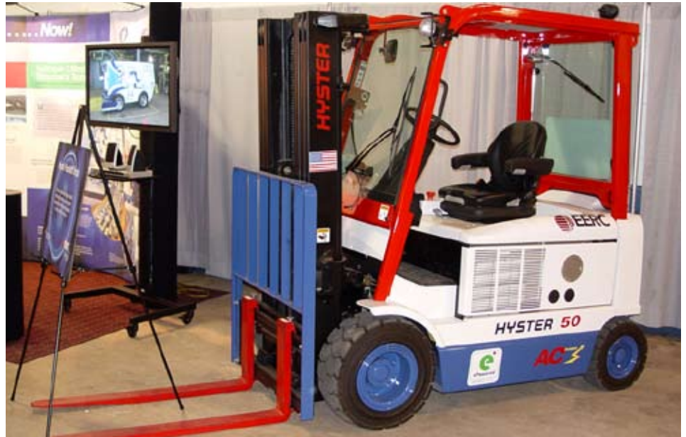
The EERC has partnered with the U.S. Army Research and Development Center, ePower Synergies, Inc., and the U.S. Air Force to develop a Hyster fuel cell-powered forklift.
