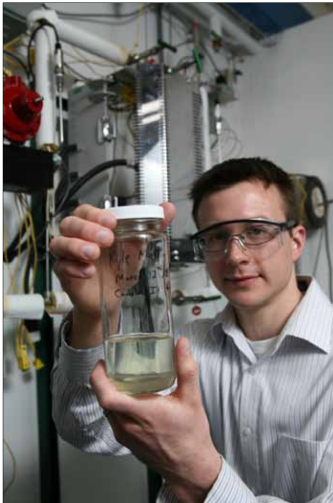
Ben Oster, a Research Engineer at the EERC, holds a sample of jet fuel made from plant oils. This fuel will be combined with coal-derived fuels made in the renovated Slurry Building to yield high-performance jet fuels.
