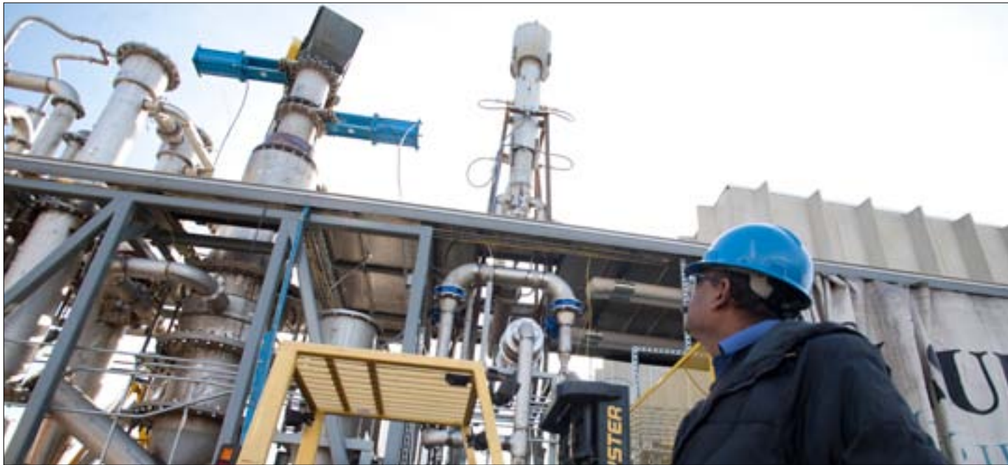
Designer Nikhil Patel observes the clean flaring of syngas during his successful first test of the semitrailer-mounted gasification unit (featured in the July/August 2011 issue of the EERC Edge) built by EERC engineers and technicians. This gasification unit converts forestry wood waste into a clean-burning syngas.
