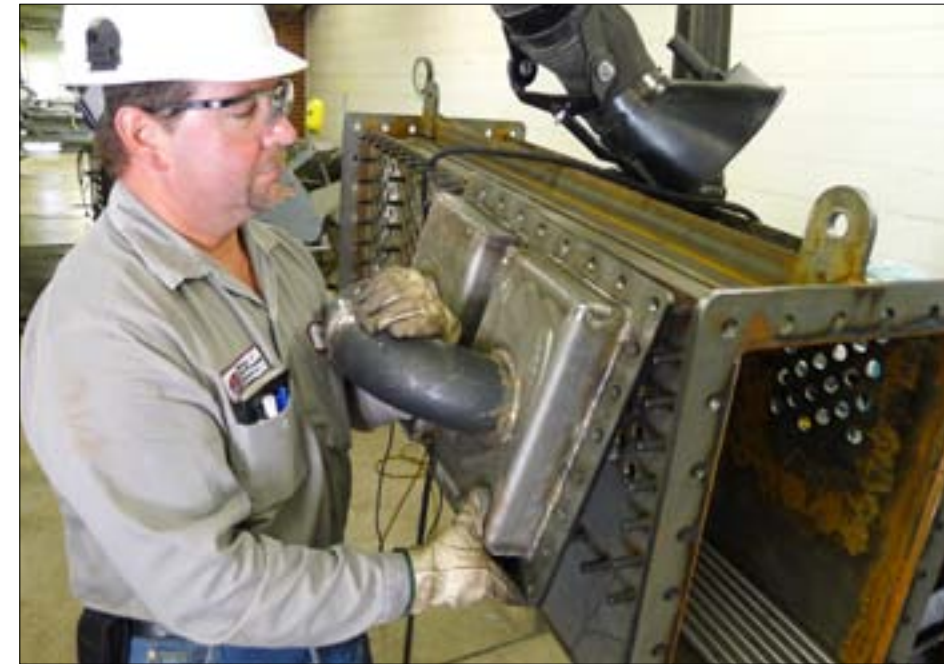
Corey Fox assembles an in-house-fabricated hybrid water condenser for a DOE-funded project studying ways to minimize water use in coal-fired power plants.
