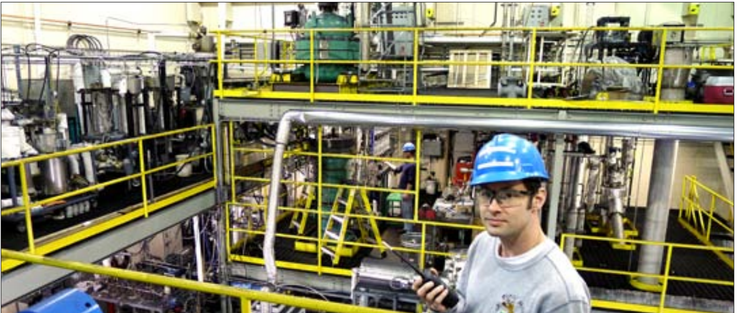
Josh Stanislawski, Research Manager, oversees operation of the EERC entrained-flow gasifier that can be used for coproduction of power, hydrogen, fuels, and chemicals.
