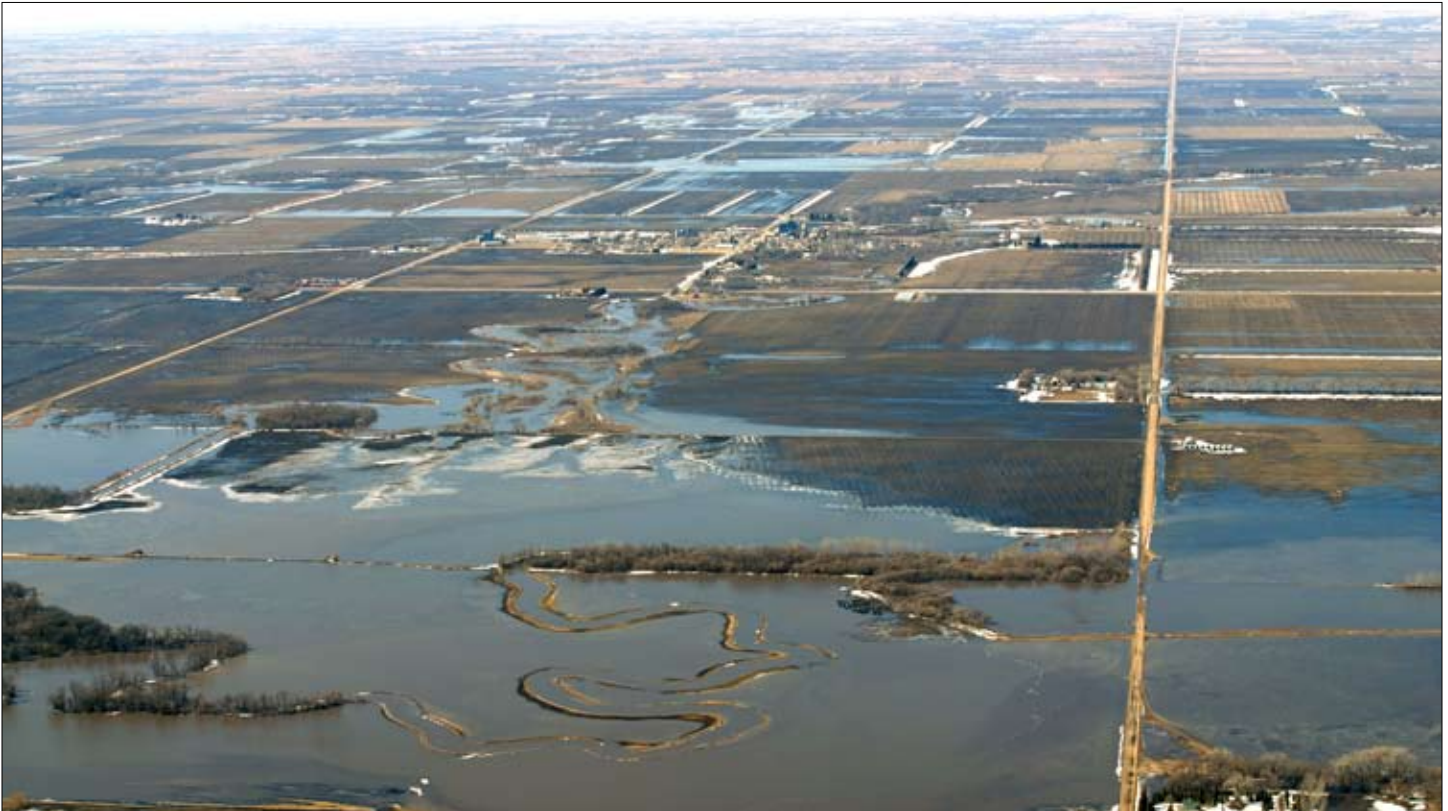
An aerial photo shows the Red River Valley during normal spring flooding in 2004. The EERC’s Waffle plan would make use of existing elevations, such as roads, and depressions, such as ditches and low-lying fields, to hold back water during spring melting to augment dikes and provide real security from flooding along the Red River and its tributaries.
