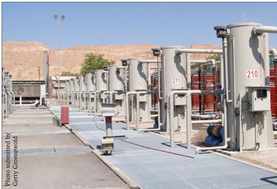
The algae facility at Kibbutz Ketura, 35 miles north of Eilat, which is at the extreme southern tip of Israel near the Red Sea. The Algatech biotechnology company cultivates pure cultures of the algae in a controlled, closed system and then transfers them to a modular tubular system exposed to long hours of natural sunlight for the final reddening process.
