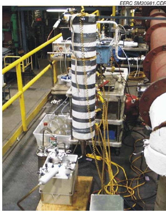
Figure 5. Entrained-Flow Reactor Sampling Real Flue Gas on the EERC Combustion Test Facility
