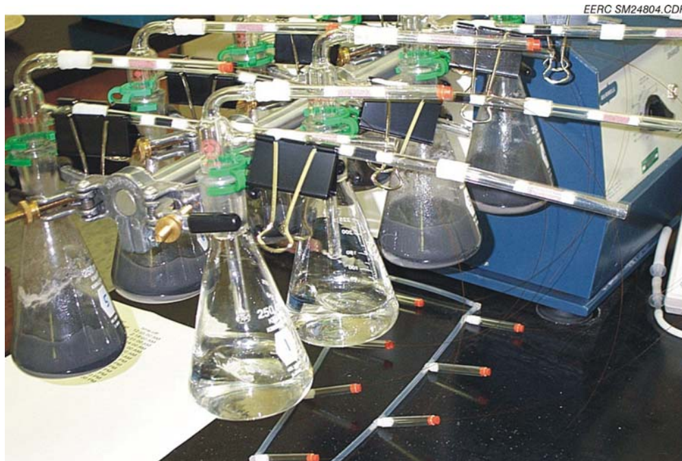
Figure 9. Microbiologically mediated mercury vapor-phase collection apparatus utilizing a wrist action shaker to facilitate mixing.
