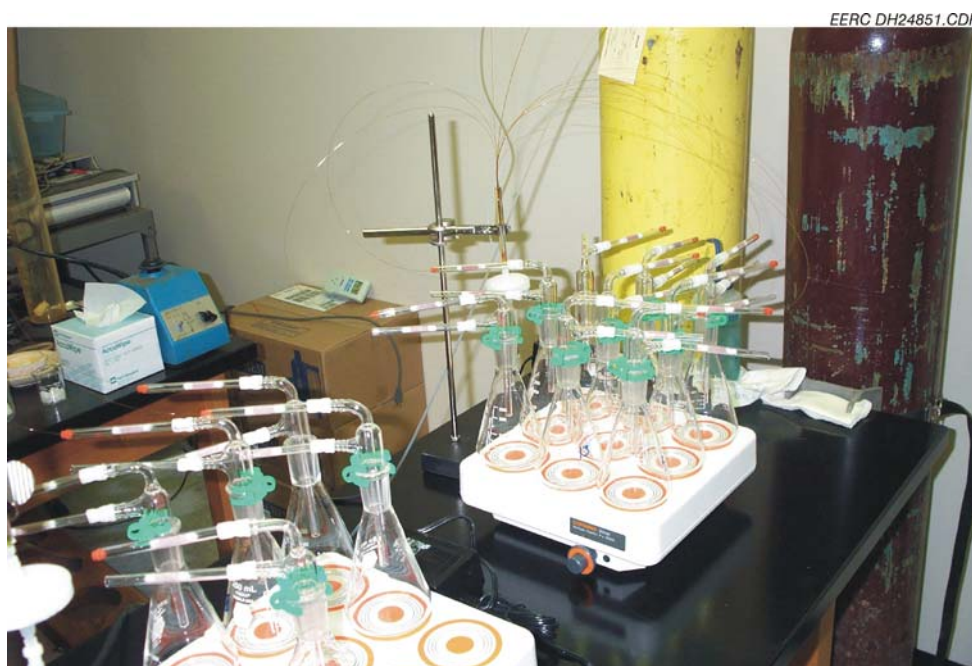
Figure 10. Microbiologically mediated mercury vapor-phase collection apparatus utilizing a stir plate to facilitate mixing.
